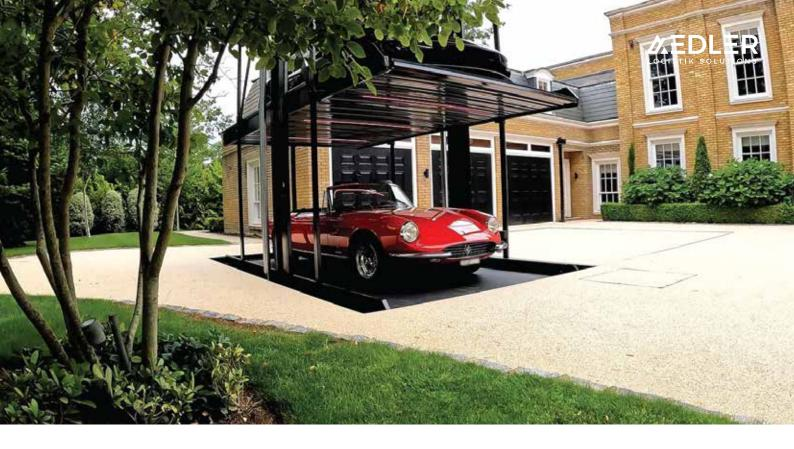
Mechanical systems are hydraulic systems with horizontal platforms designed for vertical stacking. This two-level car parking system can be designed with or without a pit and operate in both outdoor and indoor applications and is the perfect solution for space-constrained locations.
